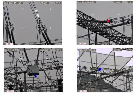
Fig. 5-8. Corona discharge in real power grids.
