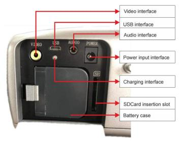
Fig. 15. Arrangement of ports under the cover.
