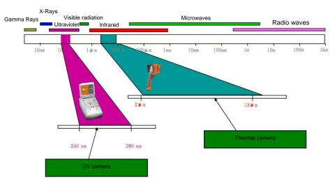
Individual types of electromagnetic radiation have wavelengths as shown in Figure 1.
