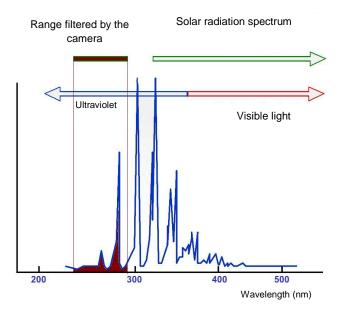
Fig. 2: The spectrum of corona discharge
